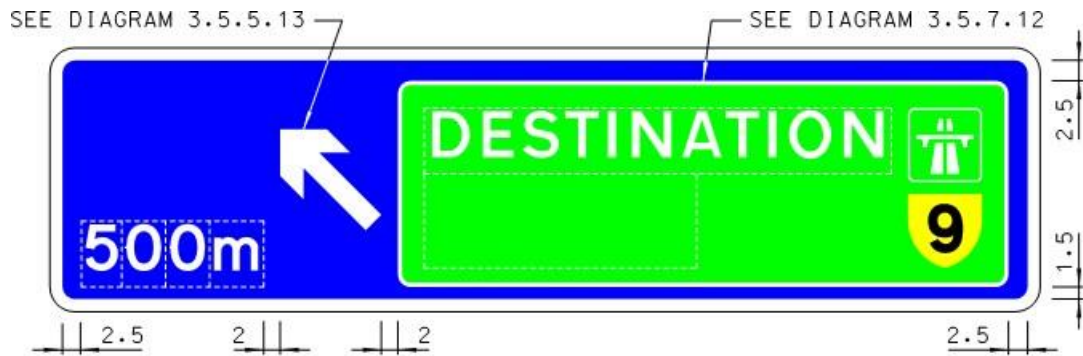
(i) ADVANCE DIRECTION SIGN
