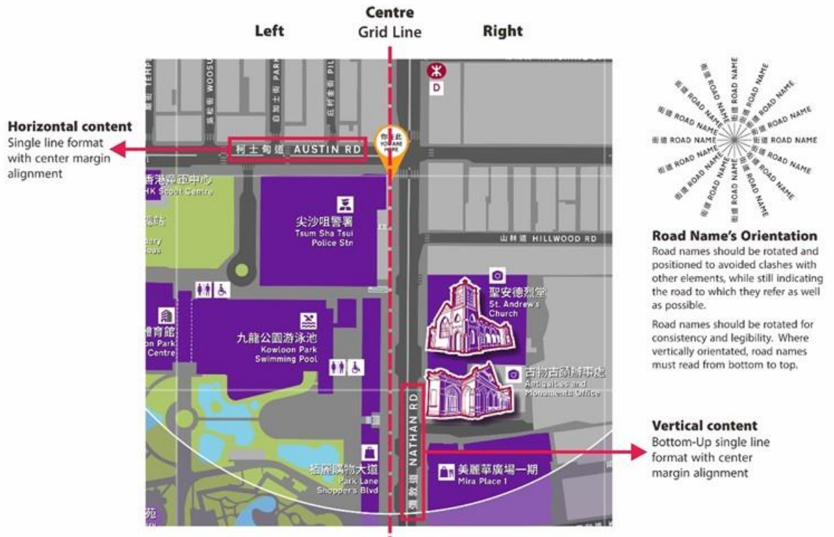
DIAGRAM 7.3.2.10 : ROAD NAME ALIGNMENT ON FOCUS MAP
