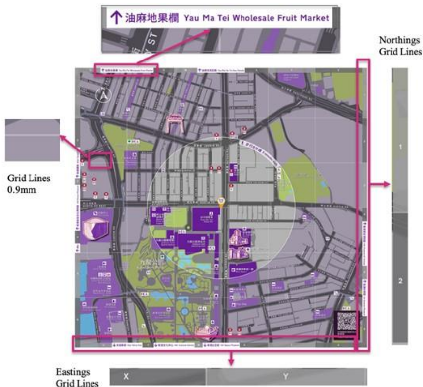
DIAGRAM 7.3.2.15 : LAYOUT OF GRID
