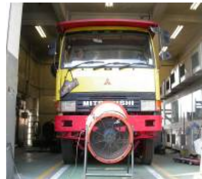
A Goods Vehicle Being Tested on a Dynamometer
